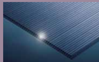
A 板材表面没有共挤UV，经照射看不出有明暗特征。 No UV layer, no silver line under UV flashlight.
