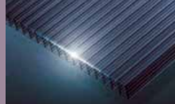
B 采用强光手电对板材横截面进行照射，与板材其它部分相比，UV层会变得明亮许多，仿佛板材表面镀了一道银边，且能清晰的看出UV分布是否均匀。 The UV layer becomes brighter than other part under UV flashlight. You can even see how thick and flat the UV was coextruded through the silver line.
